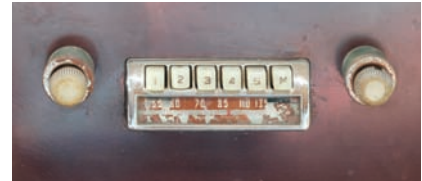
In an old fashioned radio, pushing down one station button released the others.
